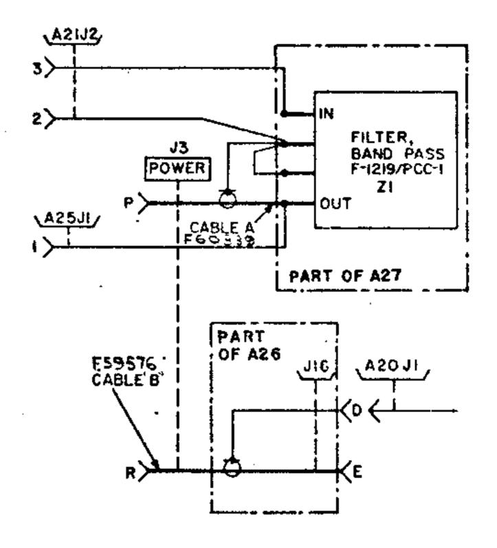
Figure 4. Receiver-Transmitter, RT-505/PRC-25, Modification Schematic
