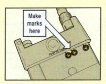
Make an etch mark on each module opposite the "O" on the dial.
