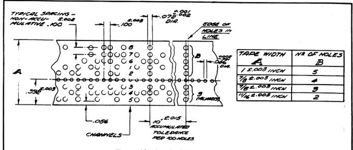
Figure 11. Standard Tape Dimensions
